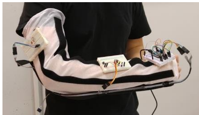
Figure 6: Wearing the Tortillaboard prototype. At this point, the user can relocate their widgets as they see fit.
